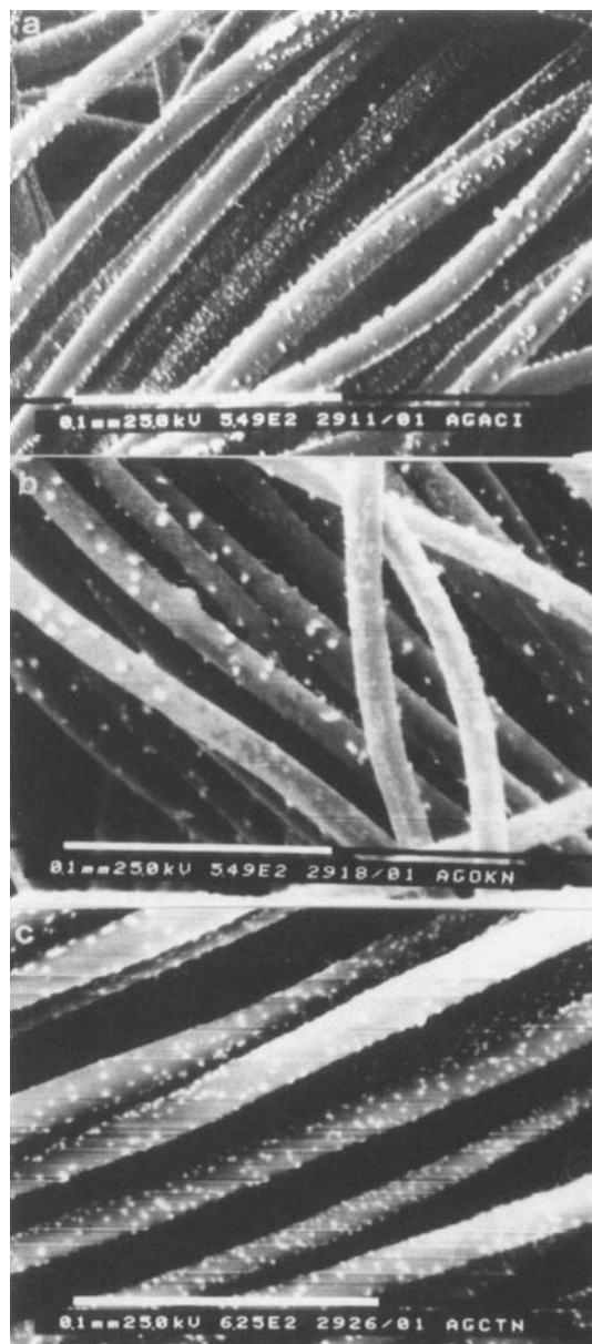
FIG. 5 Micrographs of samples impregnated with silver salts, magnification 549\times : (a) ACC + Ag(I) acetate, (b) ACC + Ag(I) oxalate, (c) ACC + Ag(I) citrate.
